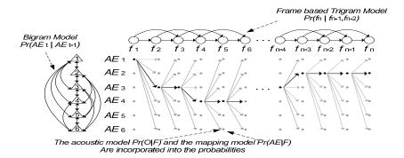
Fig. 1. Viterbi decoding algorithm
