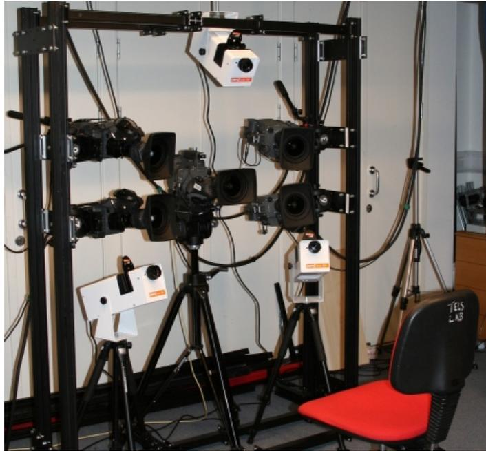
Figure 7.2: The capture setup for facial performance consists of four HD film cameras in two vertical pairs and three light projectors with colour filters. The central camera is auxiliary and is not used in the processing.
